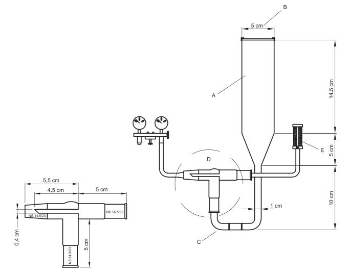
Figure 2.9.41.-1. - Fluidised-bed apparatus
