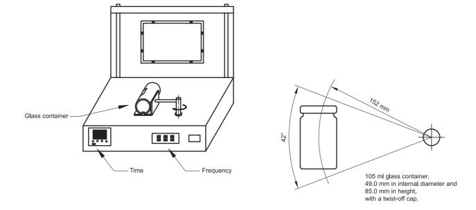
Figure 2.9.41.-2. - Oscillating apparatus
